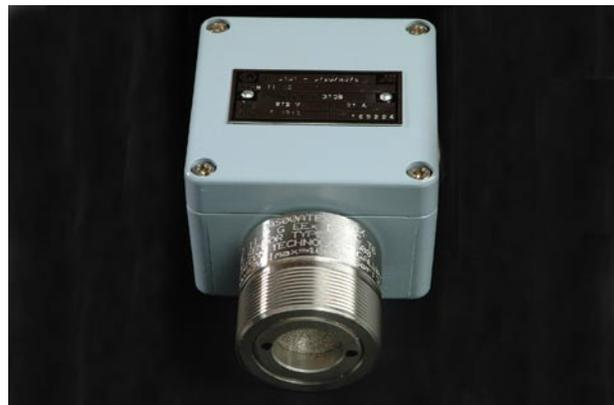
An electric current is passed through the elements which raises the temperature to a level where oxidation will occur. The catalyst reduces the temperature at which oxidation occurs, thus prolonging the life of the elements and resulting in much lower power consumption.
