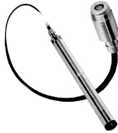
The MJK Expert™ Log 900 Level Logger is battery powered with a built-in data logger. It is designed for level and temperature recordings in wells, bore holes and storm flow locations over longer periods. It has an external diameter of 22 mm and is made of 316L stainless steel.
