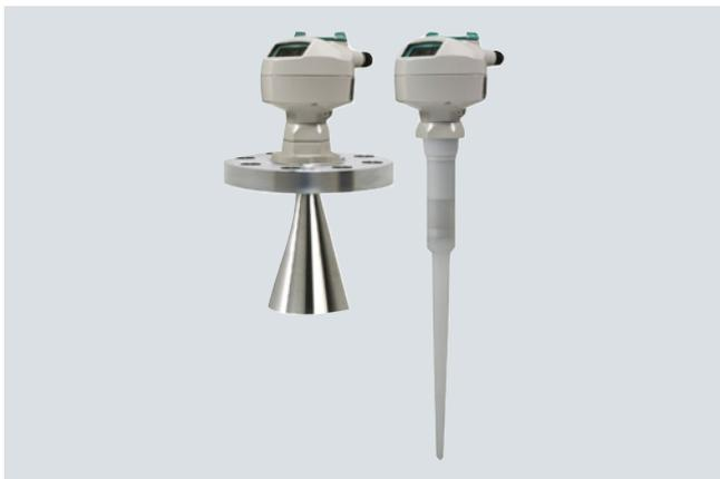
SITRANS LR200 is a 2-wire, 6 GHz pulse radar level transmitter for continuous monitoring of liquids and slurries in storage and process vessels including high temperature and pressure, to a range of 20 m (65 ft).
