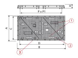
Made of ductile iron. Fulfils the requirements of European standards EN-124.
