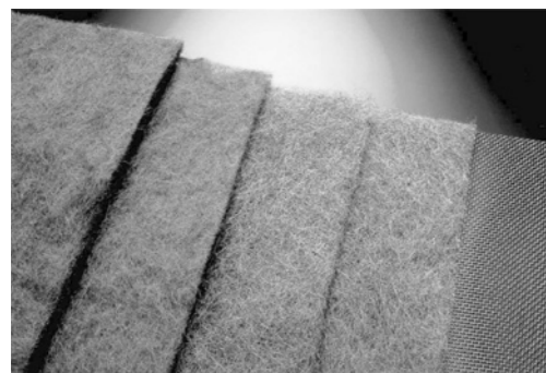
Stainless steel fleece for depth-filtration
