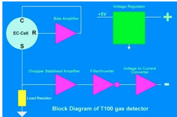
The T100-HCL is a 4-20mA, 2-wire transmitter to measure a hydrogen chloride gas in the range 0-30ppm and 0-50ppm. It is housed in a rugged, compact metallic enclosure. It incorporates advanced SMT electronics and an amperometric electrochemical sensor based on micro fuel cell technology, designed to be maintenance free and inherently stable.
