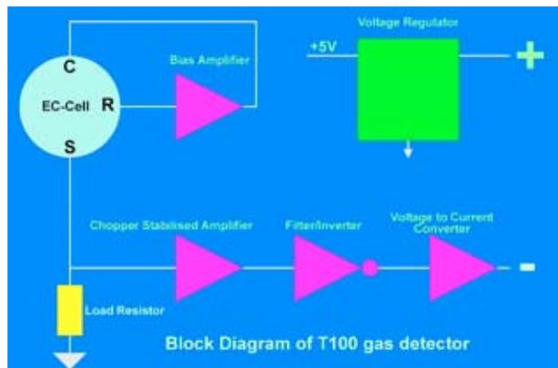
The T100-COCl<sub>2</sub> is a 4-20mA, 2-wire transmitter to monitor phosgene gas in the range 0-5ppm (other ranges are also available to special order). It is housed in a rugged, compact metallic enclosure. It incorporates advanced SMT electronics and an amperometric electrochemical sensor based on micro fuel cell technology, designed to be maintenance free and inherently stable.
