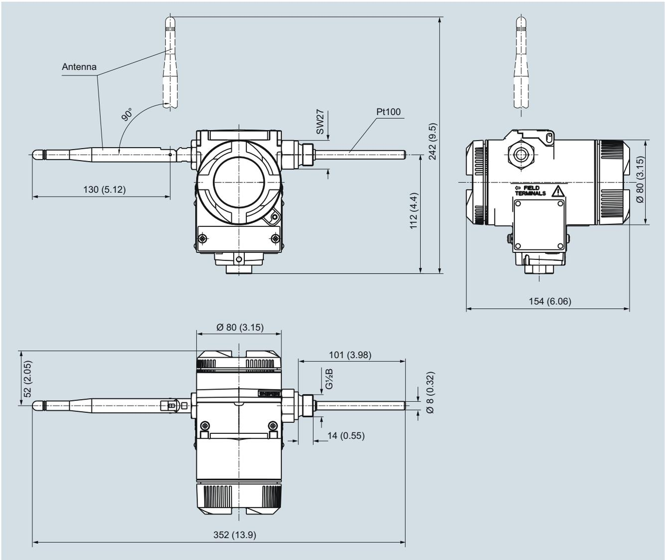
SITRANS TF280 WirelessHART temperature transmitter with Pt100, dimensions in mm (inch). Please see the dimensional drawing of the mounting bracket on page 1/192.
