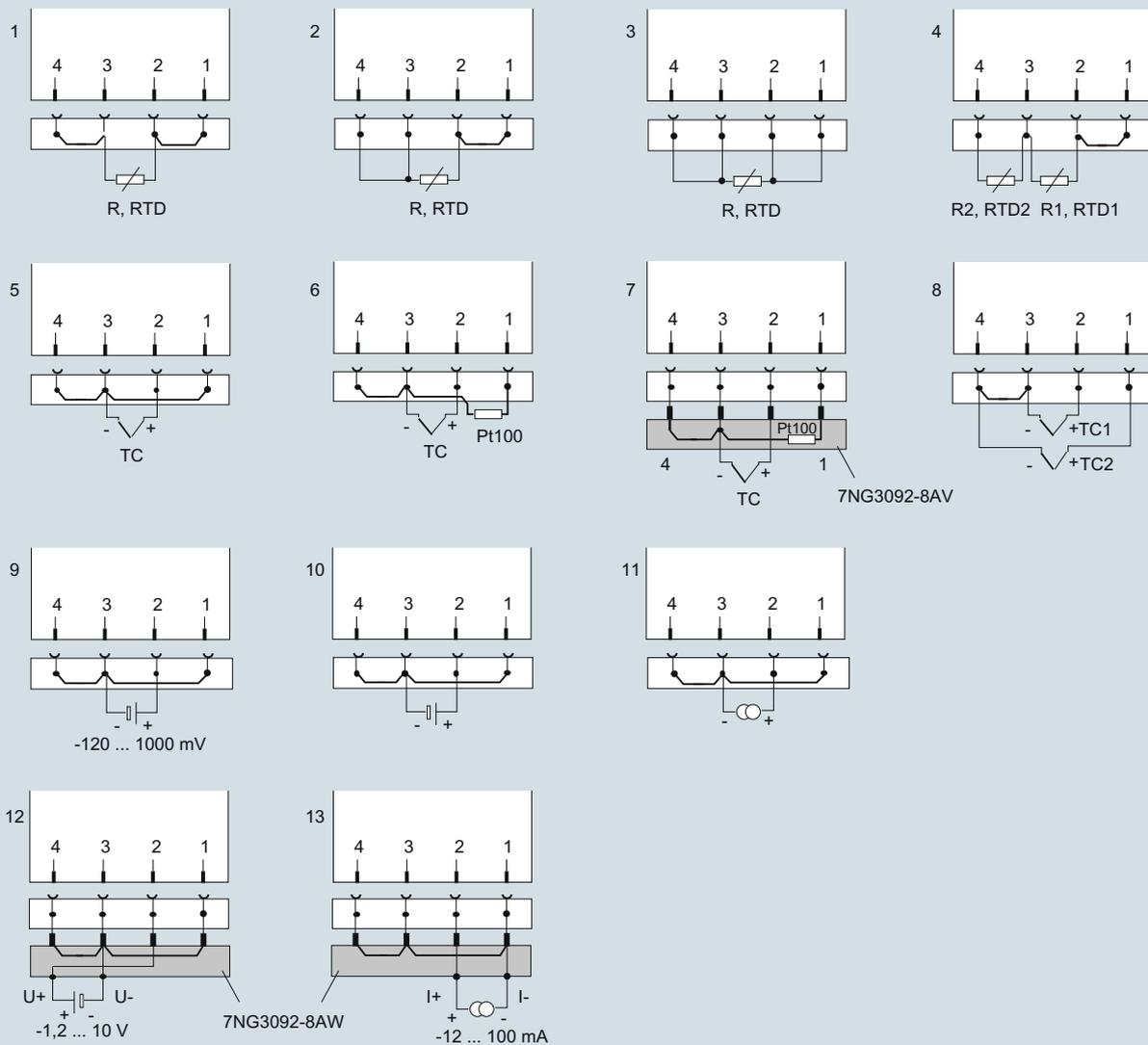
Resistance thermometers, resistance-based sensors, potentiometers:
