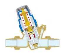
The pressure reducing valve AQUA 80-451 is supplied with compensated seats. This means that the calibrated pressure value downstream remains constant regardless of changes to upstream pressure. In the figure, the thrust towards opening is counterbalanced by the closing pressure acting on the compensating piston. As the latter has a surface area equal to that of the obturator, the two forces cancel each other out.
